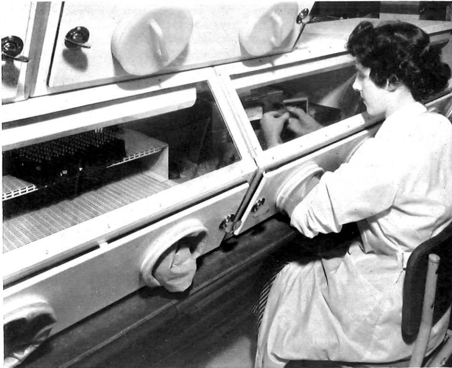
A girl operator at the Mullard works in Southampton assembles a transistor inside a dust-free humidity cabinet.
