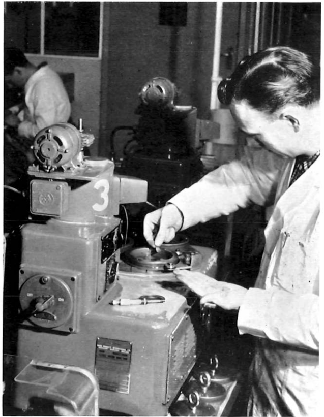
Slices cut from a bar of purified germanium are lapped to reduce their thickness. Later, the slices are etched in baths of acid.
