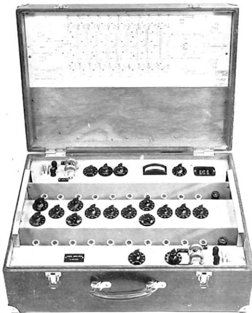
A No. 98A amplifier which was developed by the Post Office in the early 1950s. It was more portable than the previous type of telephone pair repeaters.
