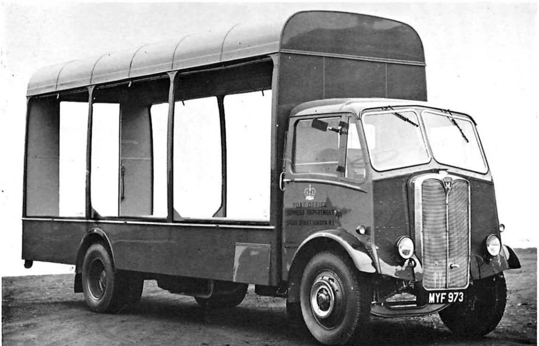
Fig. 2: Vehicle fitted all round with roller shutters to facilitate palletized loading
