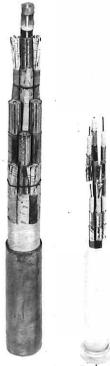
Fig. 1: 0.375" 4-tube and 0.163" 6-tube coaxial cables
