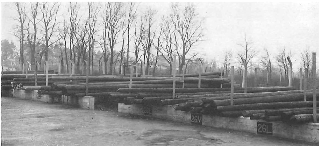
Fig. 6: Pole stack stagings with concrete walls
