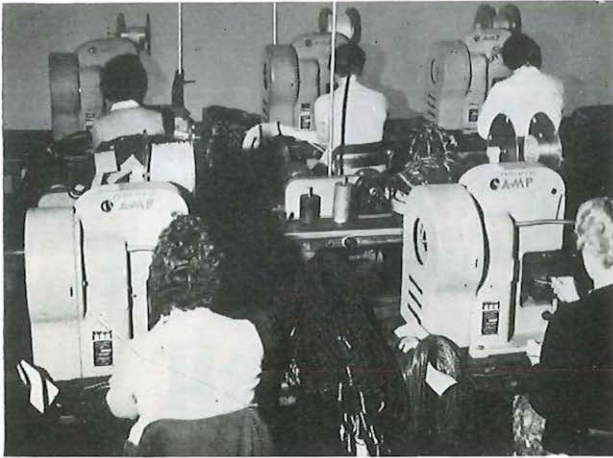
The above illustration shows a battery of Automachines applying spade terminals to telephone cords
