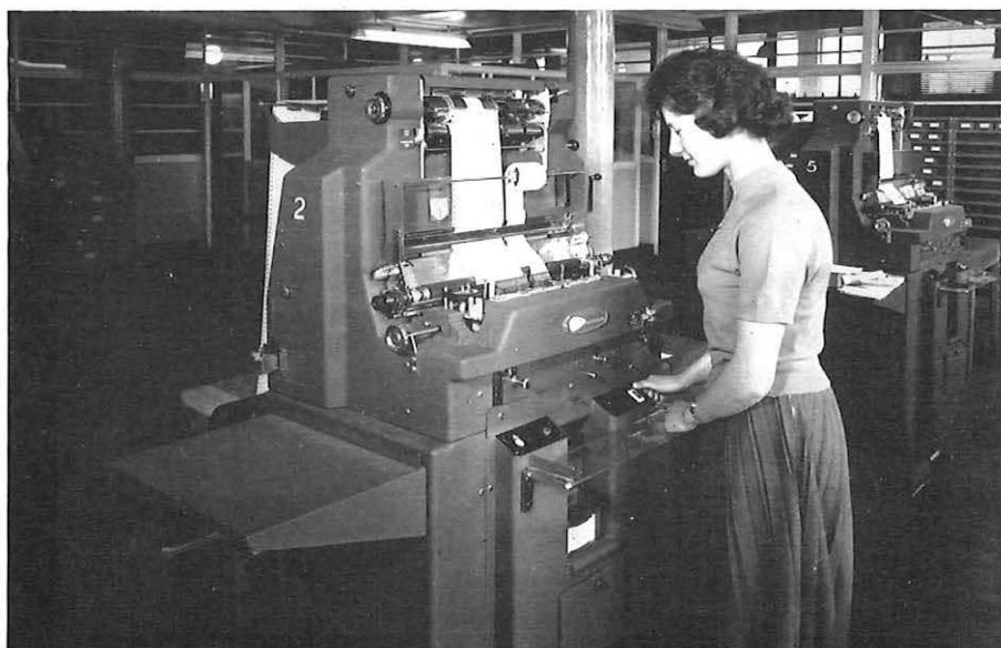
Fig. 3: A punched-card tabulator producing trunk statements at the Manchester ticket processing unit (Courtesy, JCT Ltd.)
