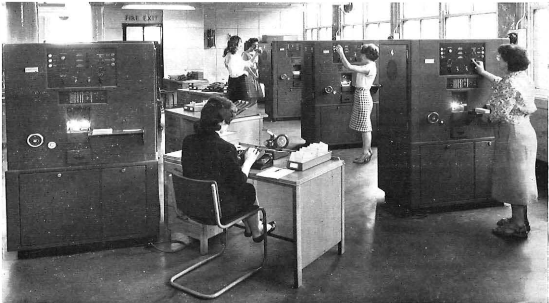
Fig. 2: Mark-scanners at the Manchester mechanical ticket processing unit
