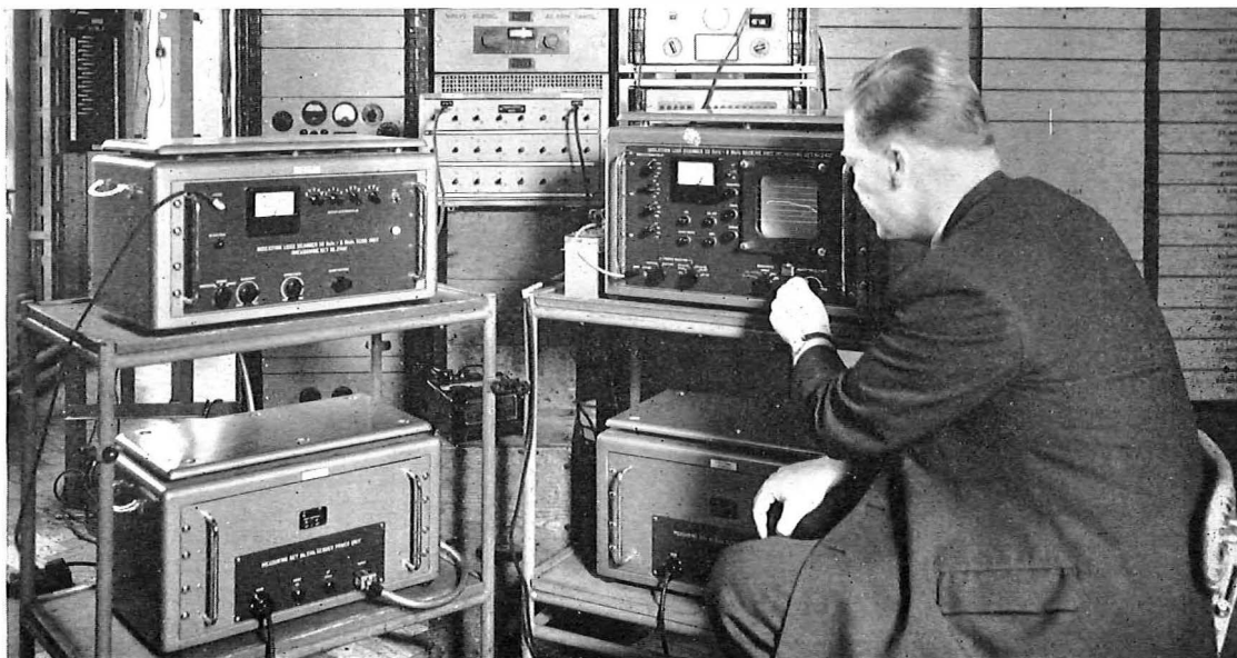
Fig. 2 (below) : Insertion loss scanner displaying loss/frequency response of equalized coaxial line link
