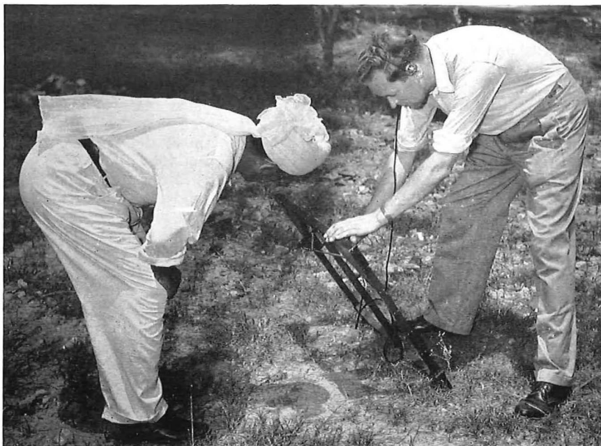
The author demonstrates the use of a cable search coil to a Regional School Instructor
