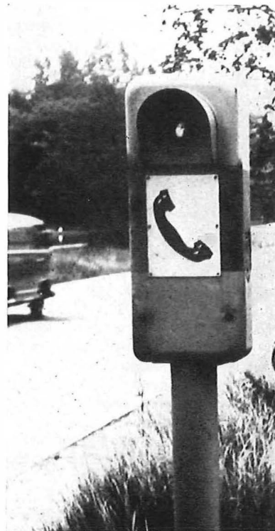
Fig. 2 : German superhighway communication Pillar (Siemens)
