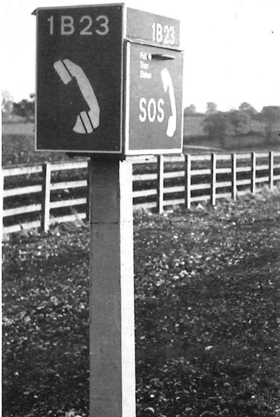
Fig. 4 (a) and (b) : Emergency telephone pillar and cabinet, designed by Ministry of Transport for M.1
