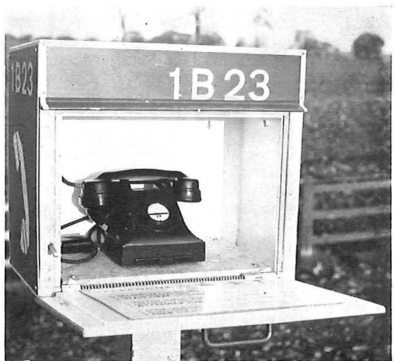
Fig. 4 (a) and (b) : Emergency telephone pillar and cabinet, designed by Ministry of Transport for M.1
