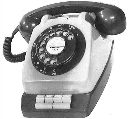
Fig. 2: Telephone No. 706 standing on a model of the 6-button plinth for Extension Plans Nos. 5, 5A, 7 and 7A
