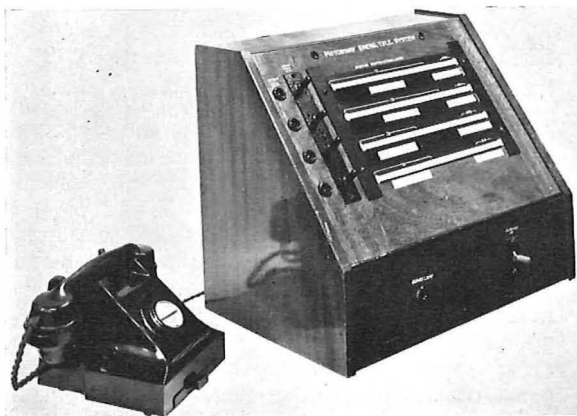
Fig. 5 (a) and (b): Table-mounted switchboard, and equipment rack, at St. Albans police station
