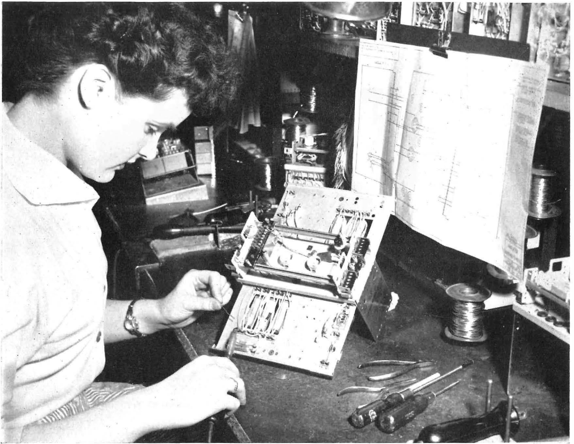
Fig. 7: Operator wiring 56-type units
