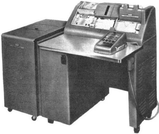
The I.B.M. data transceiver which allows direct card-to-card transmission (Courtesy, I.B.M. United Kingdom Ltd.)
