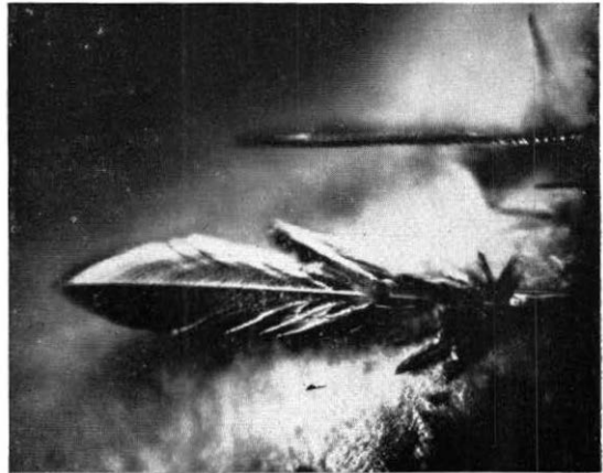
Dendritic and tapered growths on sulphide coated silver contacts (magnified 200 times)
