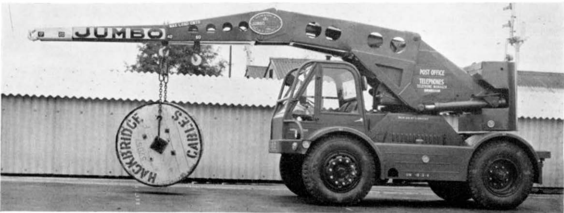
Fig. 7 below : Jumbo 3-ton crane
