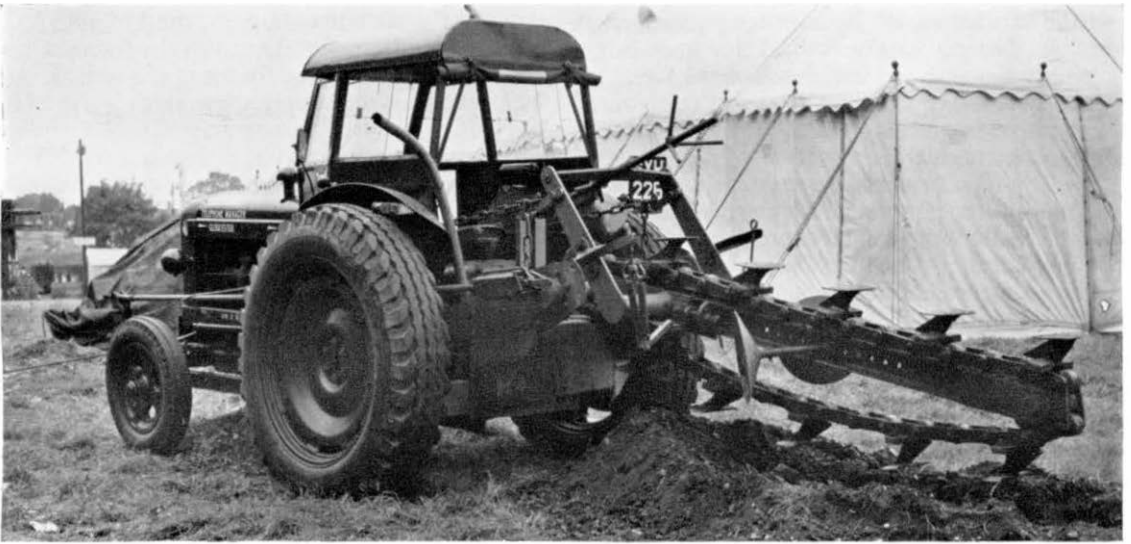
Fig. 5 : Astell-Watts trench excavator
