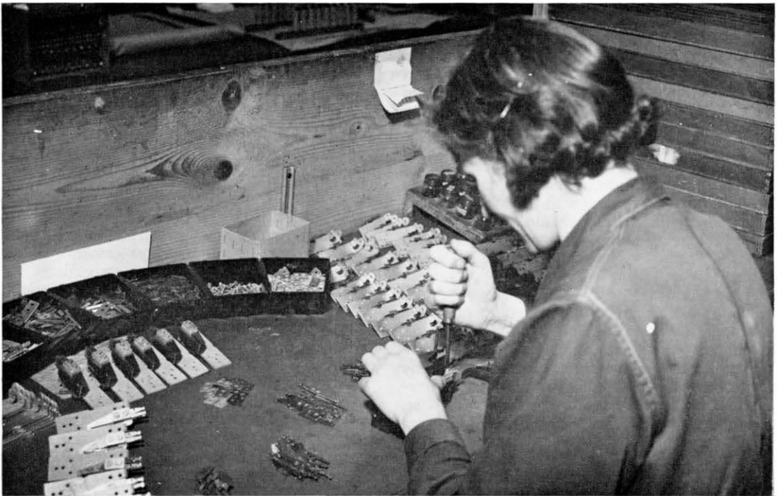
Fig. 6 : Assembly of Strowger type spring sets
