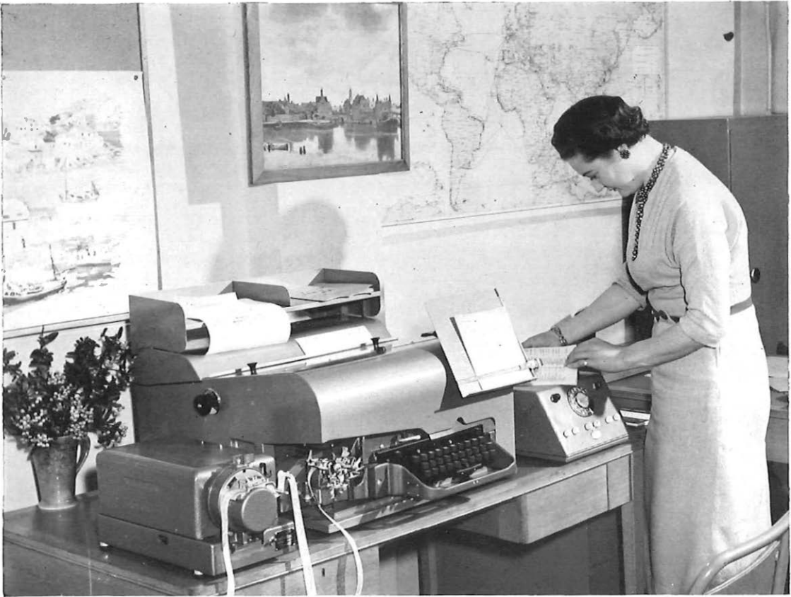
Installation with reperforating facilities and automatic transmitter—mounted on office table
