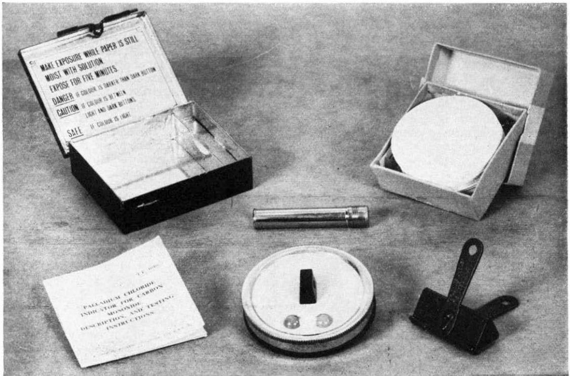
Fig. 1: Gas Leak Indicator No. 2
