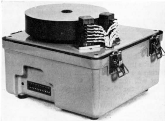
Fig. 4: Magnetic drum for recording oral announcements
