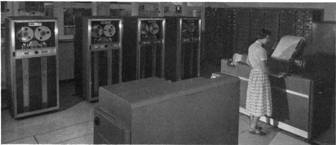
Fig. 5 : Backing store with four machines for reading and writing magnetically (Courtesy, I.B.M., Ltd.)
