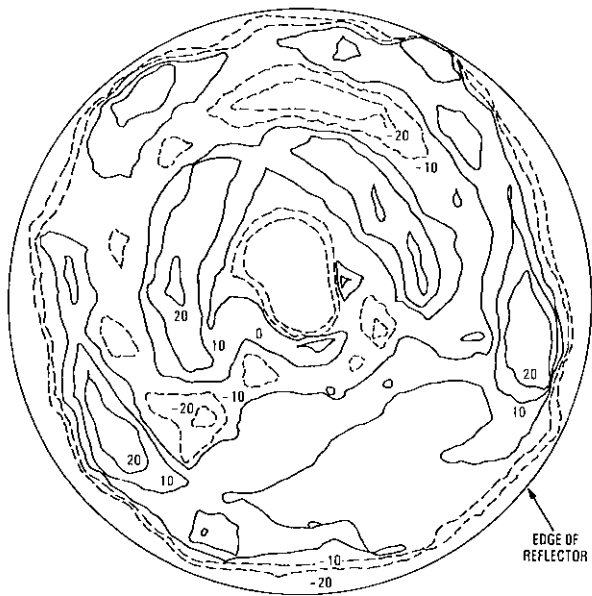
FIG. 10—Profile contour for Goonhilly 3 after fitting the subreflector
