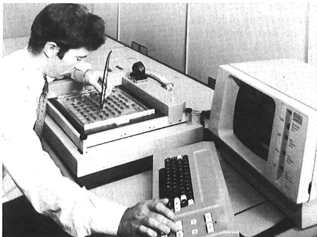
FIG. 4—Automatic fault isolation using guided-probe technique
