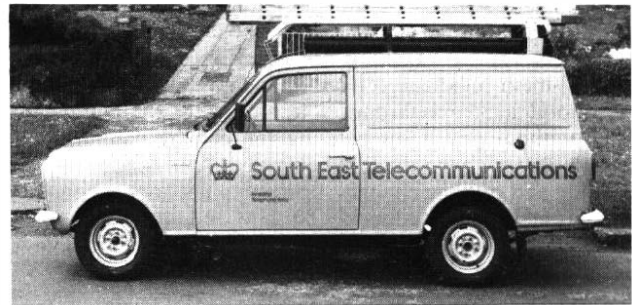
Note: This type of vehicle is used for 20 different occupations in the BPO telecommunications business, but the great majority are used by customer-apparatus and line-maintenance staff and by installation fitters. On the current field trial, the ladder rack has been raised to allow long items to be carried on the roof in PVC duct
