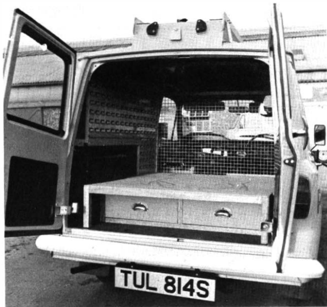
FIG. 13—A 7 cwt van fitted with a false floor unit
