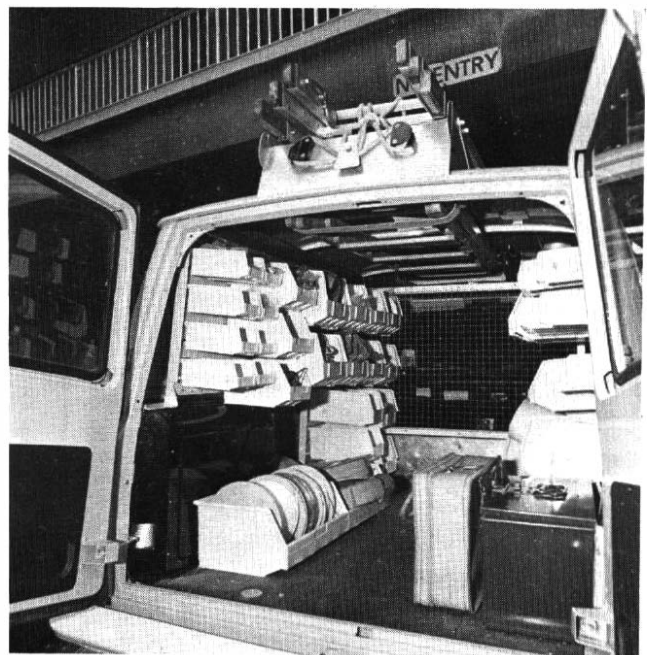
Note: The vehicle shown has been kitted out with the new standard louvred panels, together with the standard kit of plastic bins (BPO Kit No. 344A), tools and stores for this occupation
