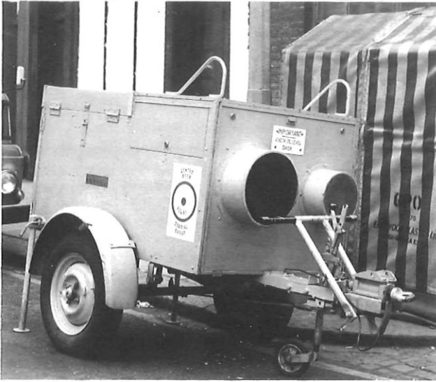
Self-contained trailer-mounted generator
