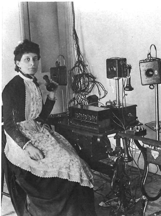
FIG. 2—The Blake microphone and the Bell earphone (In use at the Croydon telephone exchange in 1884)
