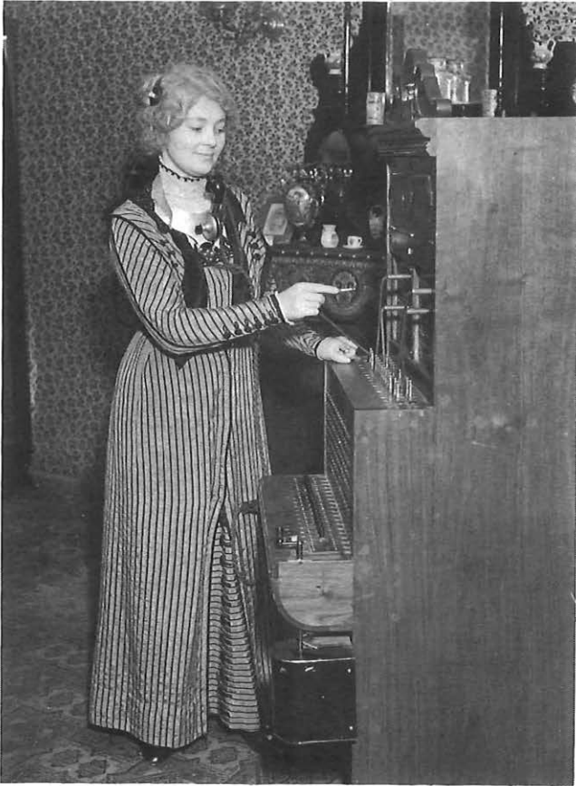
FIG. 3—The Ericsson head-and-breast set, c 1908
