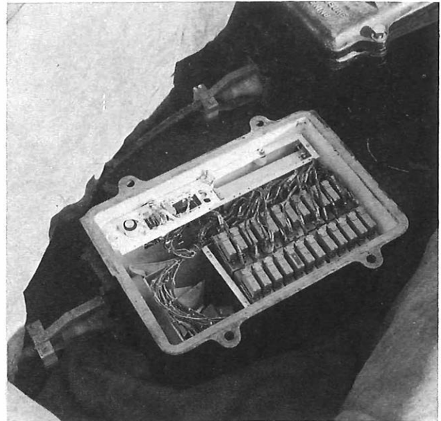
FIG. 23—Partially-equipped repeater case
