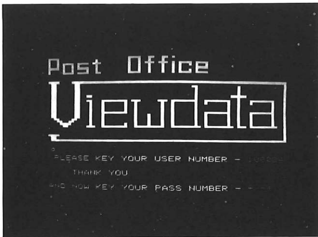
FIG. 7—First frame transmitted by a computer once a user has established contact with the Viewdata system
