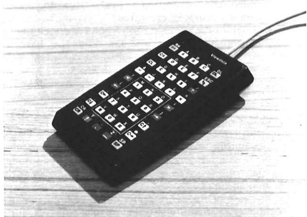
FIG. 3—Keypad having facility for message transmission
