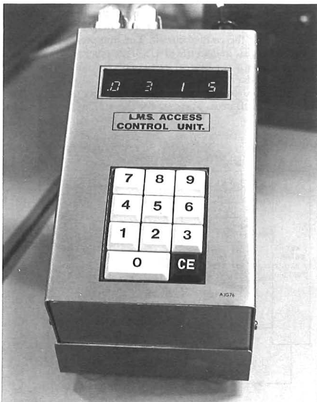
FIG. 4—Access control unit
