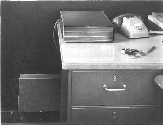
FIG. 2—Table-mounted modem unit with wall-mounted line unit
