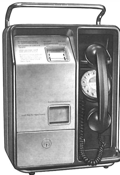
FIG. 2—New portable CCB (CCB No. 725) attached to tubular-steel frame (front and rear views)
