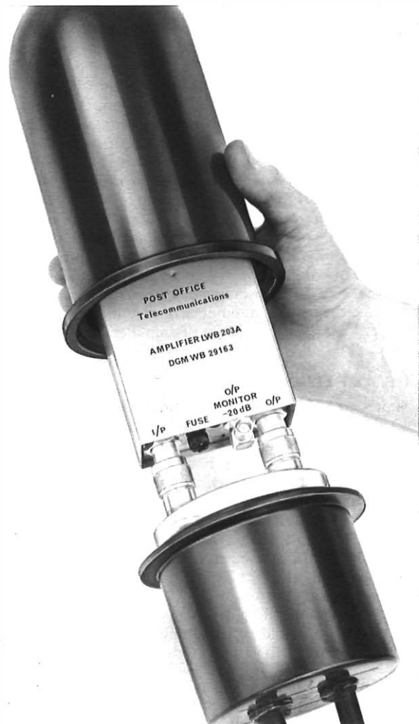
FIG. 4—Third-generation VHF-UHF amplifier in Sleeve No. 31A
