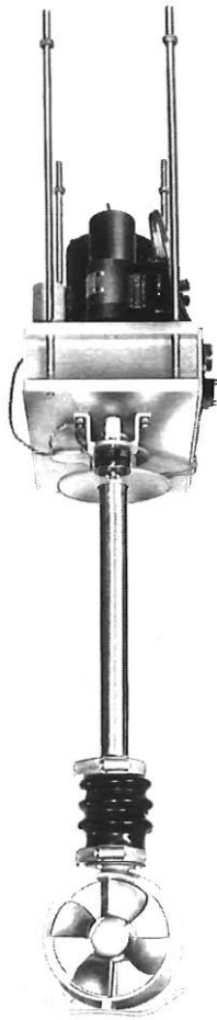
FIG. 5—Model of bow-thrust unit
