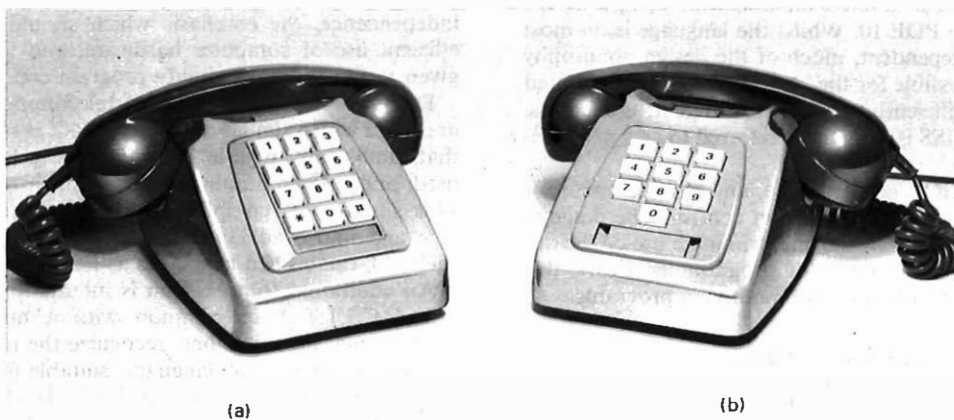
(a) Multi-frequency and d.c. code C signalling instrument (b) Loop-disconnect signalling instrument
