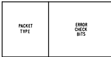
FIG. 5—Loop-delay-measurement packet structure
