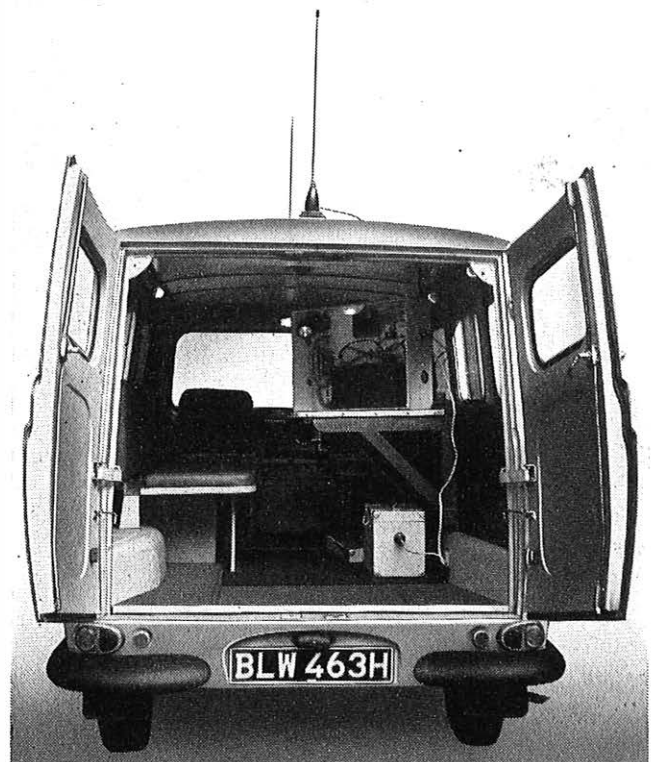
FIG. 2—An emergency radiophone unit ready for use in a vehicle. Sufficient table space is available for two units to be operated simultaneously.
