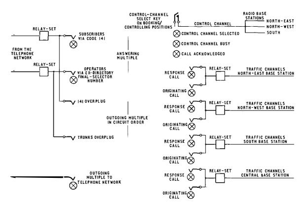
Note: All answering jacks, i.e. 141, trunks and traffic channels have a 3-panel repetition so that, when traffic is light, only one operatoris required
