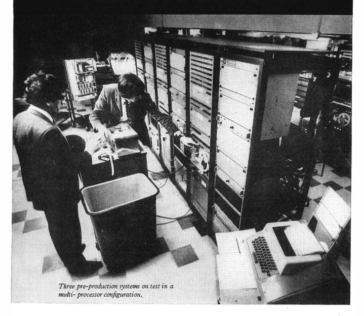
System 250 is unique. It has been designed specifically for controlling telephone and data exchanges and similar reliability-conscious real-time applications. It is modular in design in order to be flexible and easily extensible in operation and to provide economy in use.
