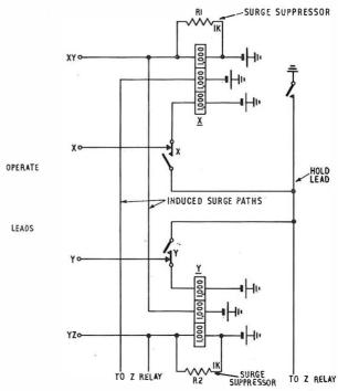
FIG. 13-Suppression of interference surges by shunt resistors
