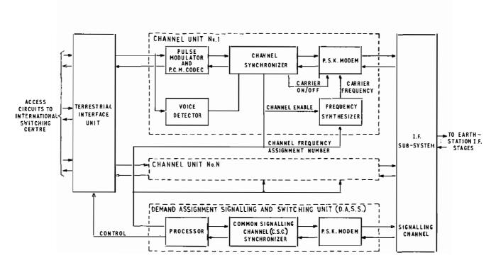
FIG. 1-SPADE system-simplified block diagram.
