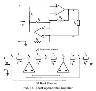
If  $Z_4$  is made a capacitor  $C_4$  and all the other impedances are resistors then the circuit becomes the preferred circuit of Fig. 15(a)
