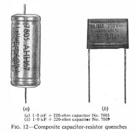
effective when connected across contacts to suppress interference from arcing and sparking. Fig. 13 illustrates an interesting application of shunt-resistor quenches, to inhibit the effect of direct interference surges between relays. Relays
