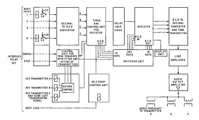
FIG. 3-Tone-generator block diagram
