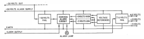
FIG. 12-Block diagram of the alarm circuit
