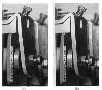
(a) Incorrect pivotting (b) Correct pivotting FIG. 21—Longitudinal overshoot of relay armature
