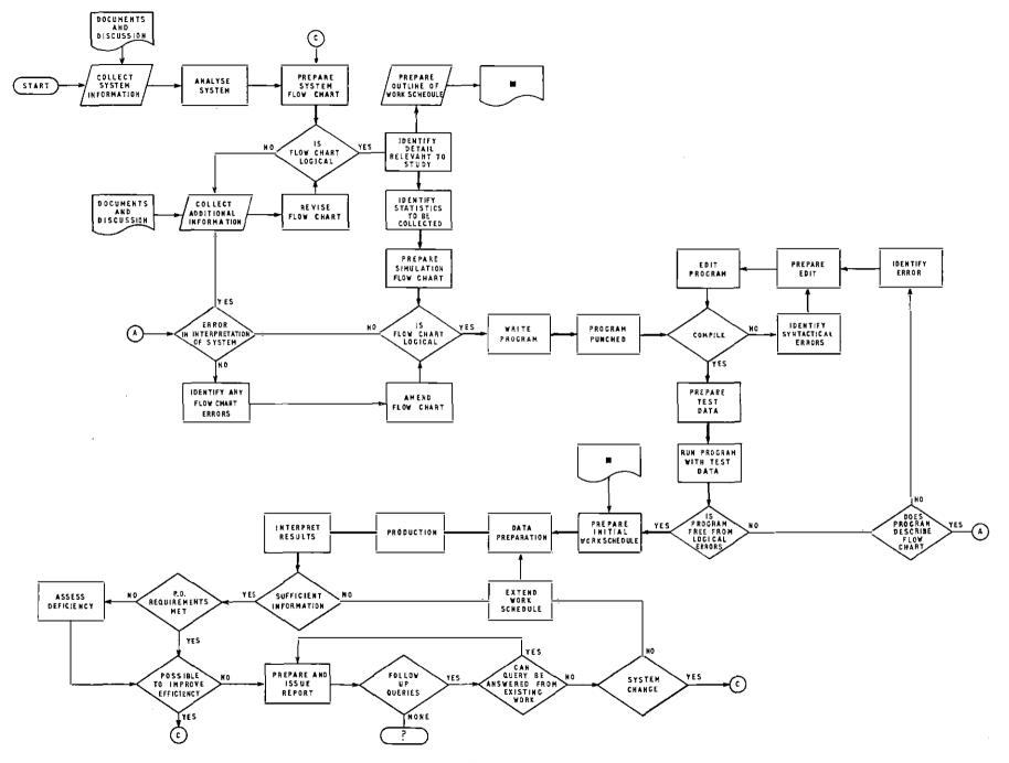
FIG 1—Flow chart of system evaluation by simulation
