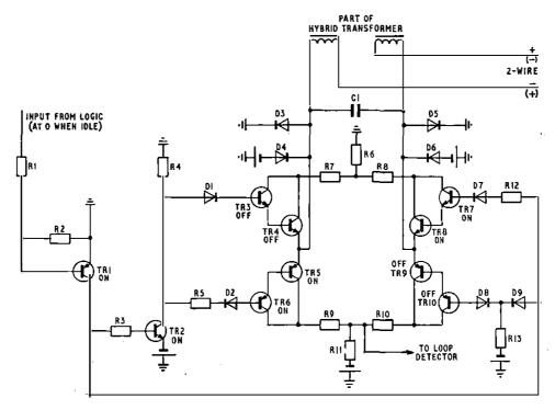
(Note: Shown in idle condition) FIG. 8—Circuit diagram of the D-relay function
