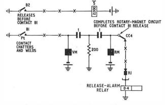
FIG. 10-Contact failure with coupled quenches
