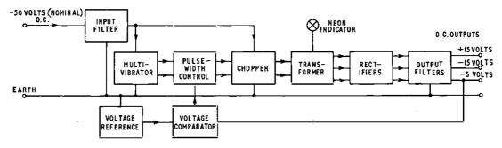
FIG. 11-Block diagram of the d.c.-d.c. converter
