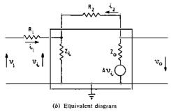
FIG. 16-Single ended inverting amplifier
