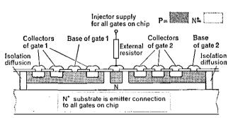
Cross-section of a pair of gates with PN injection of minority carriers
