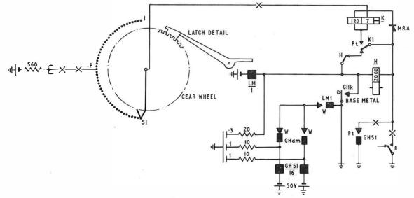
FIG. 8-Quenching of motor uniselector magnet coils
