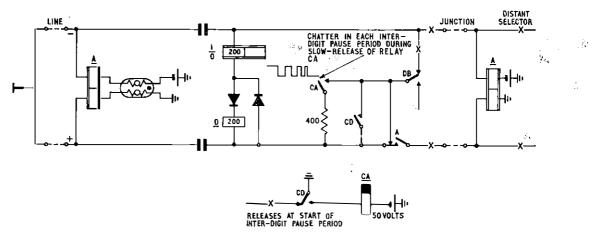
FIG. 19-Contact chatter causing noise in transmission path
