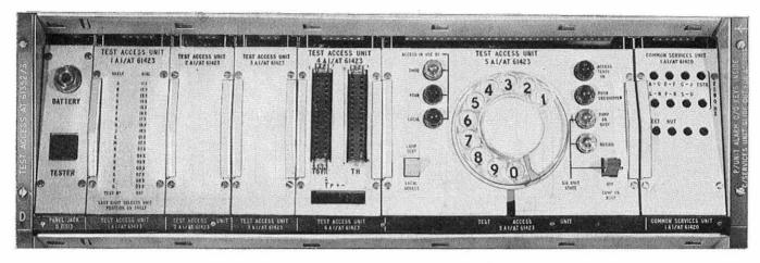
FIG. 13-Photograph of the test-access shelf
