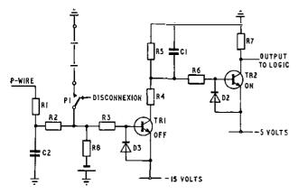
FIG. 7—Circuit diagram of the P-wire detector
