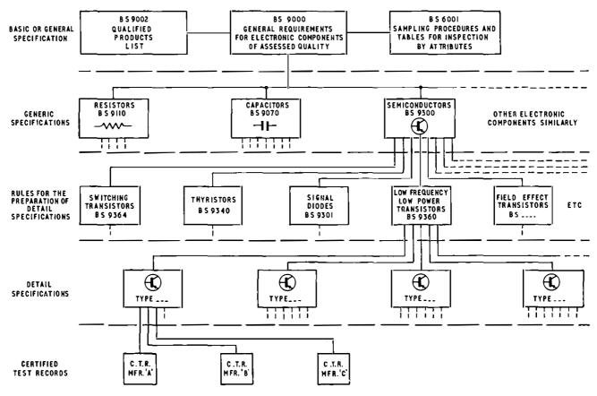
FIG. 1-The BS 9000 system of specifications
