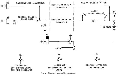
FIG. 6-Call-acknowledge and alarm-control element
