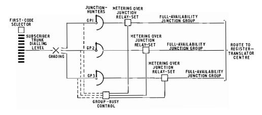
FIG. 1-Block diagram of a three-group junction-hunter scheme
