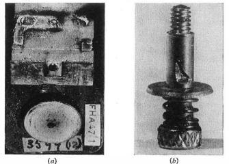
FIG. 23—Wear debris on relay knife edge and worn armature retaining screw
