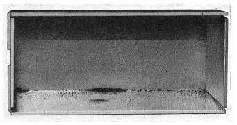
FIG. 26-Carbon particles inside dust-proof relay cover
