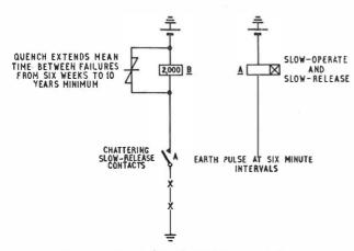
FIG. 14-Protection of chattering contacts
