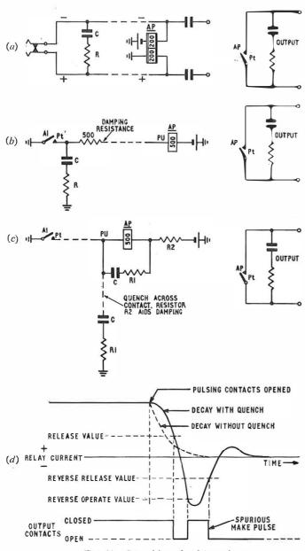
FIG. 11-Quenching of pulsing relays
