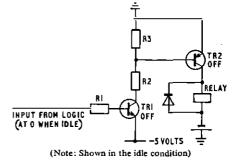
FIG. 6-Circuit diagram of the relay driver
