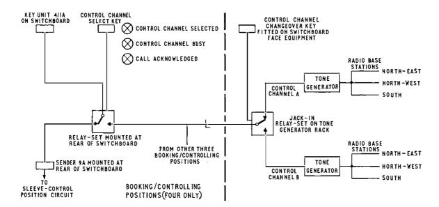
FIG. 2-Control-channel block diagram
