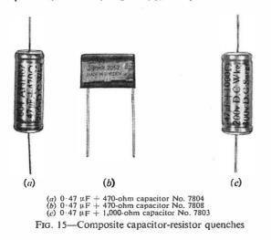
Capacitance is low to reduce erosion by inrush quench currents and avoid welding on closure. A higher resistance for platinum takes account of its greater tendency to weld.
