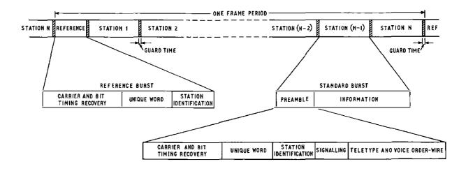
FIG. 2-Typical frame and burst format for a t.d.m.a. system.
