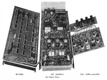
FIG. 2-Outgoing signalling unit
