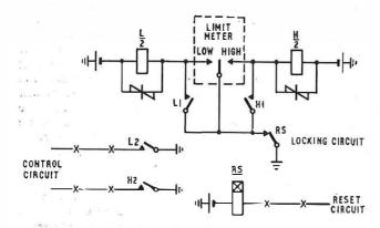
FIG. 27-Protection of limit meter contacts
