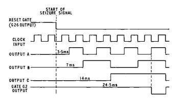
FIG. 10-Timing sequence of timer 1 (Fig. 9)
