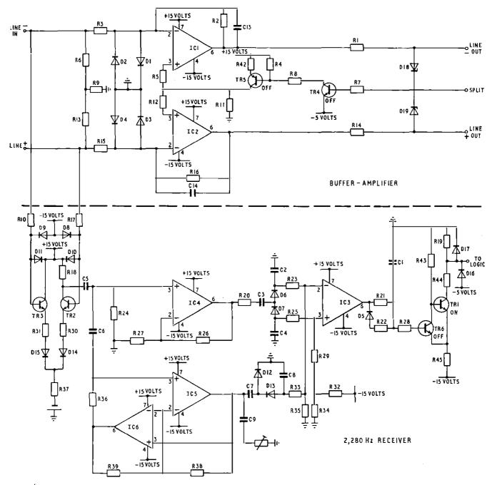
FIG. 5-Circuit diagram of the buffer-amplifier and receiver
