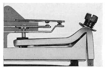
FIG. 22-Transverse overshoot and incorrect pivotting of relay armature
