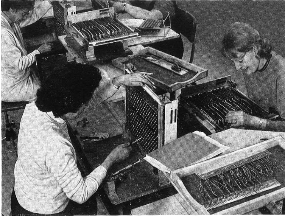
FIG. 4—Production of B-switches for TXE4 exchanges
