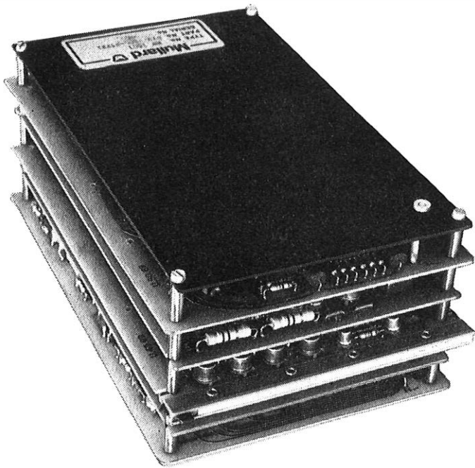
FIG. 3—The 8,192-bit ferrite core-store
