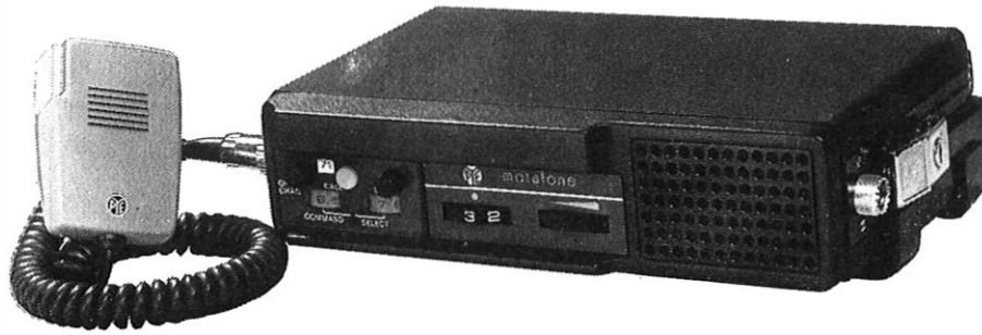
FIG. 1—Vehicle-mounted mobile-radio equipment
