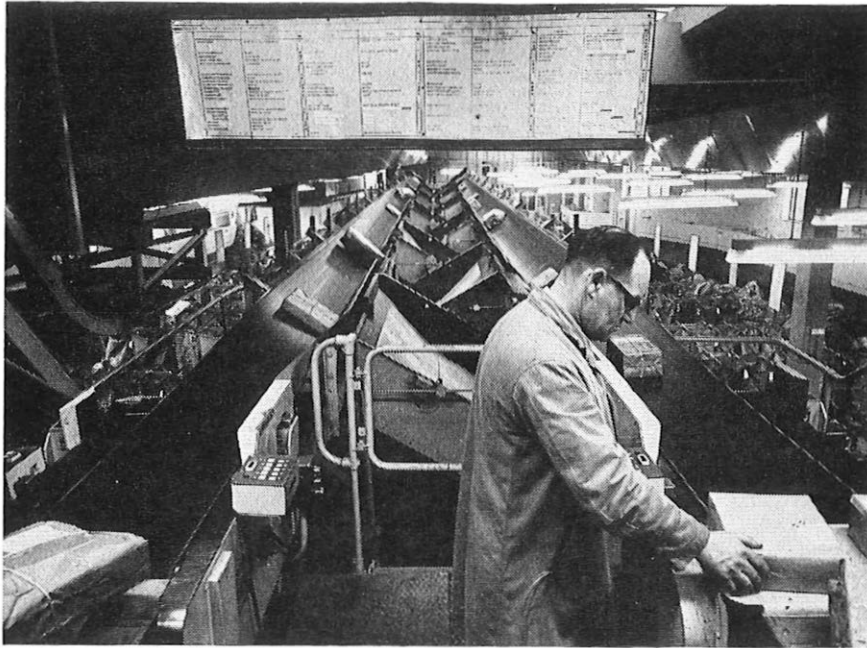
FIG 9—Tilted-belt Parcel-Sorting Machines at Worcester
