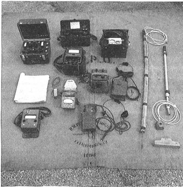
FIG. 3—Test equipment carried by external faultsmen
