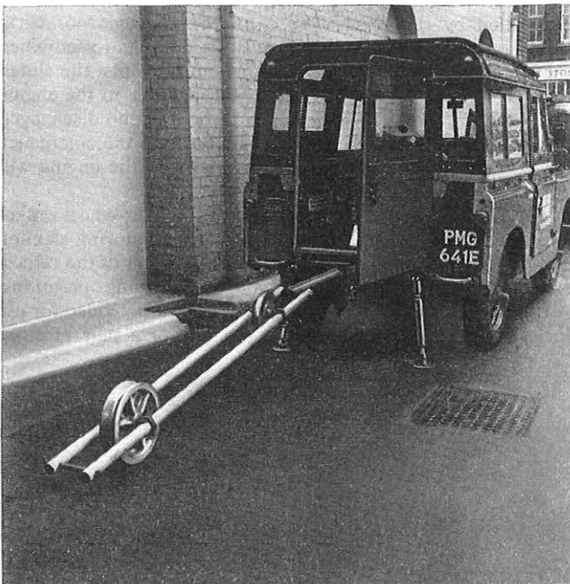
FIG. 3—Rope or cable guiding attachment anchored to vehicle by means of extension tube
