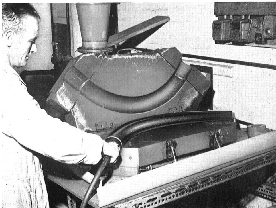
FIG. 3—Mould for production of bends
