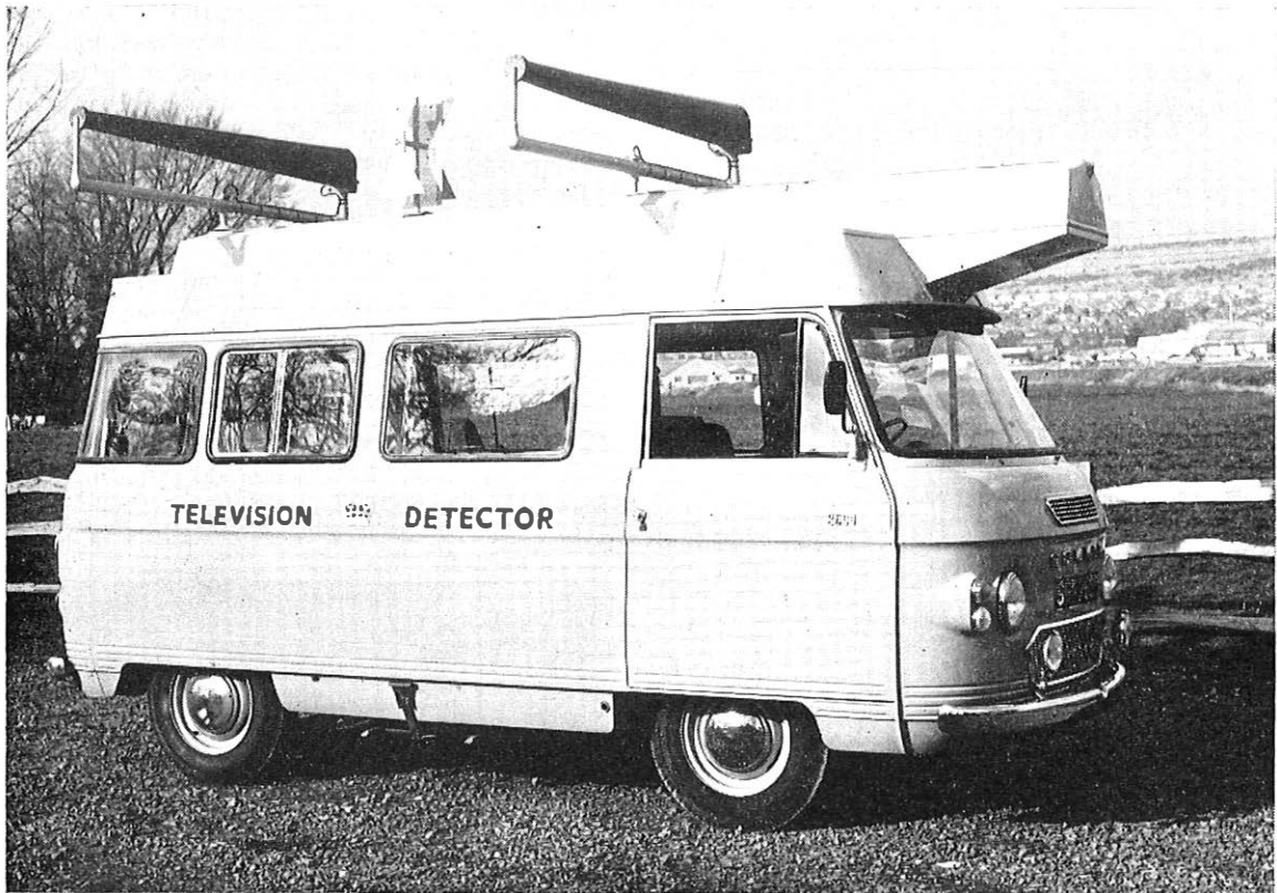
(a) The television detector vehicle showing the aerials in the operating position
