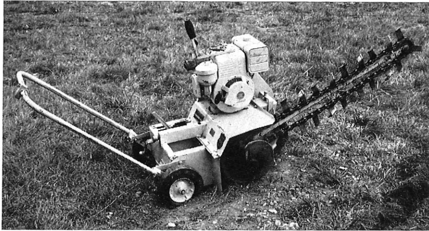
FIG. 4—TRENCH EXCAVATOR No. 1
