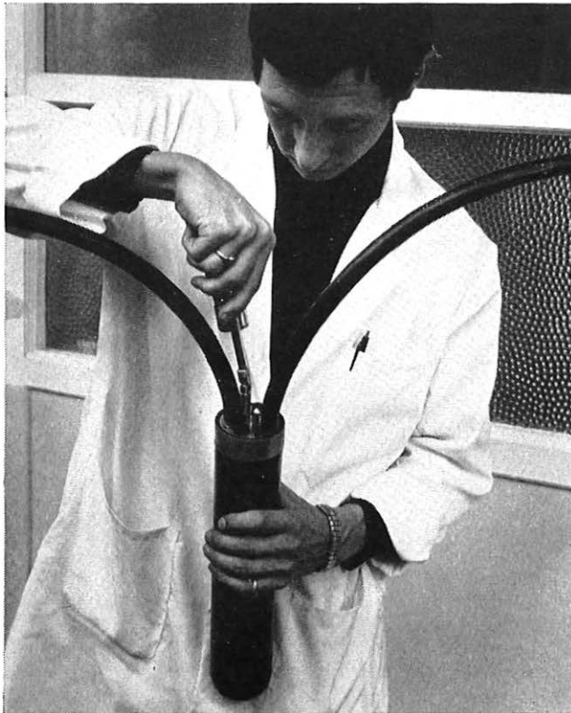
(b) Single-Ended Sleeve with Multi-Hole Expanding Plug FIG. 2—EXAMPLES OF EXPANDING-PLUG JOINTS
