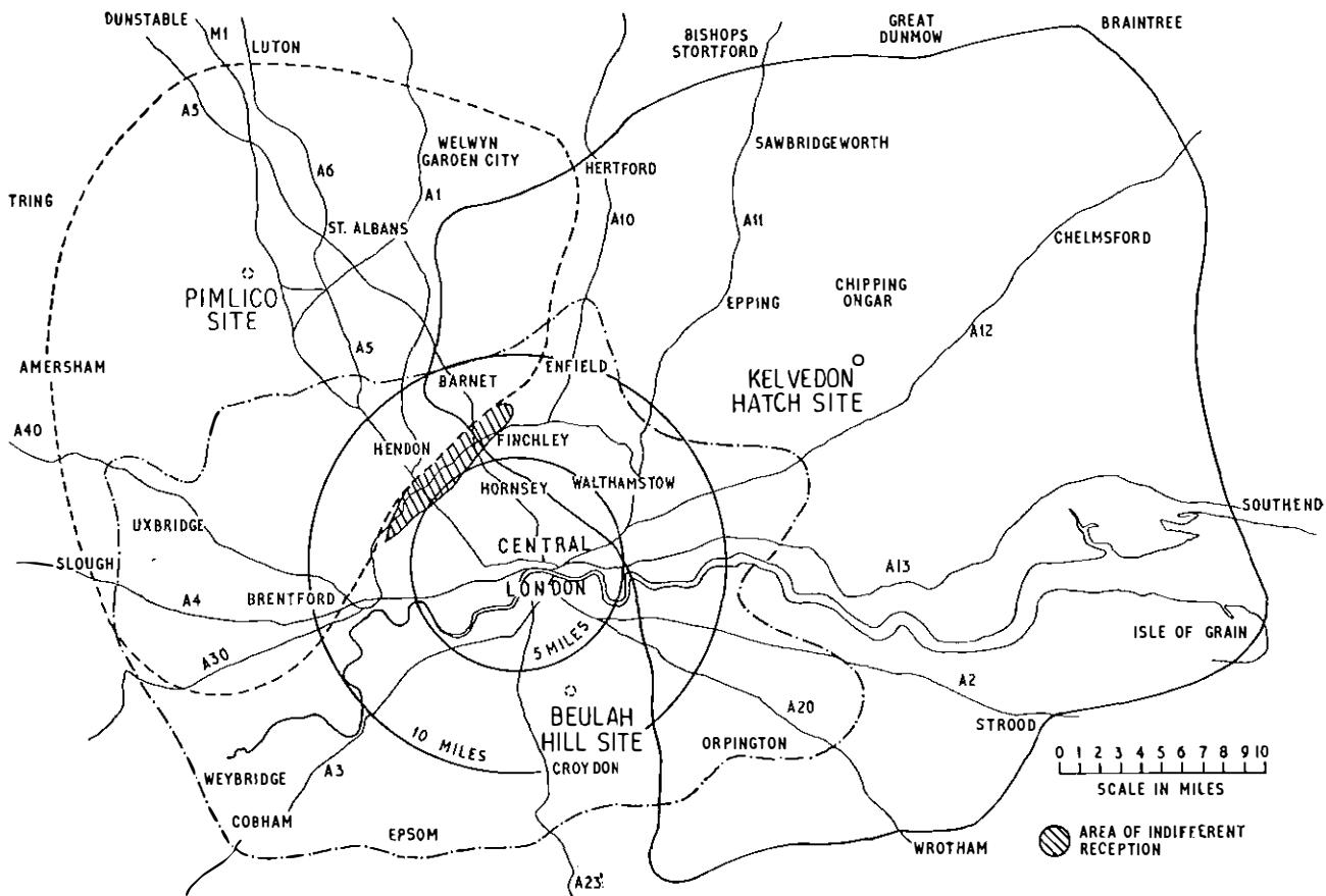
FIG. 1—SERVICE AREA OF THE LONDON RADIOPHONE SERVICE
