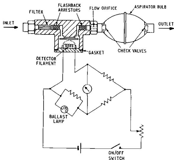
FIG. 3—SCHEMATIC DIAGRAM OF INDICATOR, GAS, NO. 5
