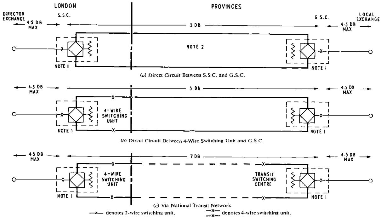
Notes 1: Exchange equipment at the S.S.C. and G.S.C. will each introduce some transmission loss but this need not exceed about 1 db.
