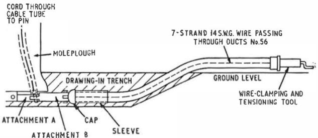
FIG. 6—EQUIPMENT READY TO DRAW IN DUCT
