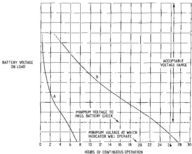
FIG. 4—COMPARISON OF BATTERY ENDURANCE FOR INDICATOR, GAS, NO. 5
