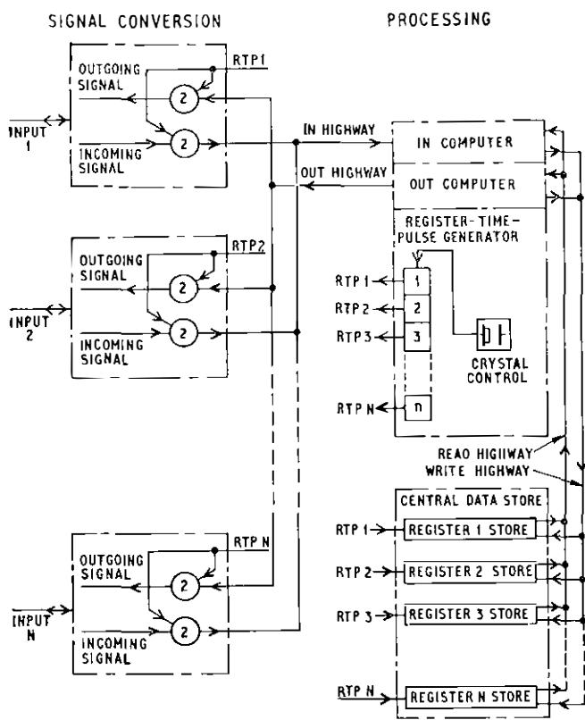
FIG. 3—SCHEMATIC DIAGRAM OF A TIME-SHARED COMMON-PROCESSING EQUIPMENT SERVING  $N$  INPUTS VIA T.D.M. HIGHWAYS
