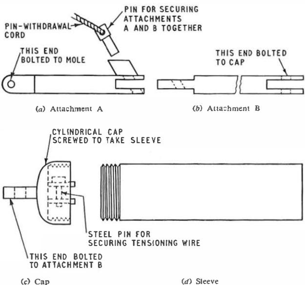
FIG. 2—SPECIAL ATTACHMENTS REQUIRED TO FIX DUCT TO MOLEPLOUGH
