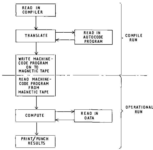
FIG. 1—PROCESSING AN AUTOCODE PROGRAM
