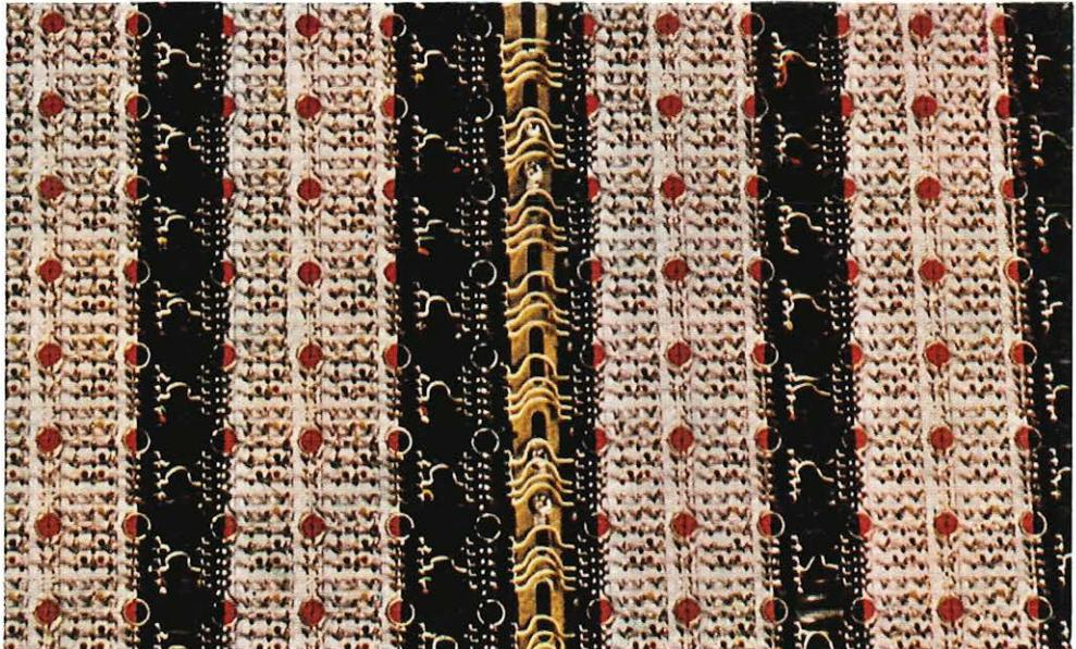
(TOP LEFT) Part of a cross-point switching frame also showing associated electronic modules.
