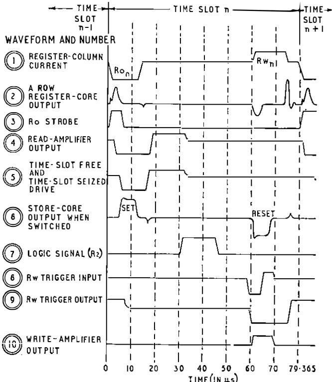
FIG. 11—CENTRAL-DATA-STORE AND FUNCTION-UNIT WAVEFORMS
