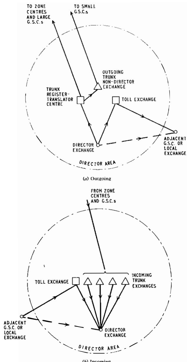
FIG. 2—PRINCIPAL EXISTING ROUTINGS FOR TRUNK AND ADJACENT-CHARGING-GROUP CALLS
