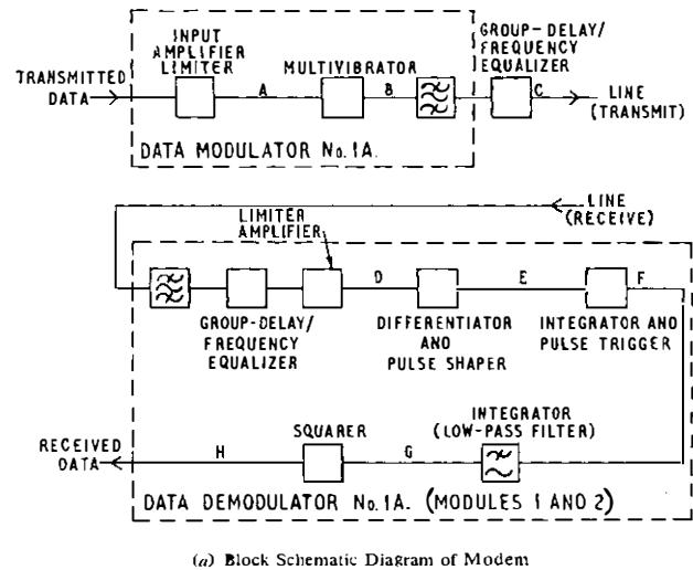
(a) Block Schematic Diagram of Modem
