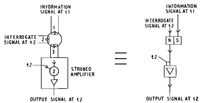
FIG. 14—THREE-WINDING-CORE FUNCTION CONTROL ELEMENT
