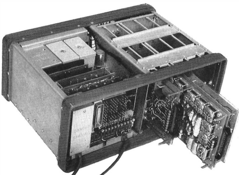
FIG. 4—DATEL MODEM NO. 1A WITH COVERS REMOVED
