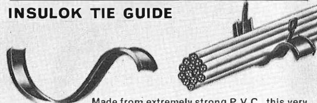
Made from extremely strong P.V.C., this very handy accessory is designed to slip smoothly between and under cable runs, permitting the easy insertion of the Insulok Cable Ties even in the most confined positions. The recessed channel guides the Cable Ties quickly and easily around any size of cable run.
