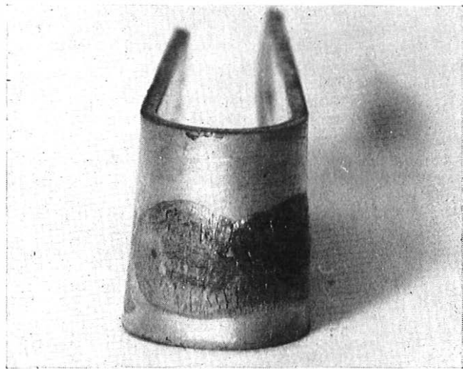
FIG. 3—CRACKS IN SOLDER ON 200-MICROINCH GOLD PLATE
