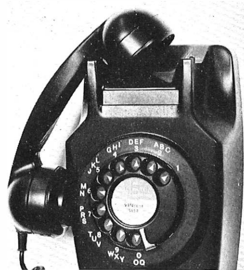
FIG. 2—"OFF-HOOK" REST POSITION FOR HANDSET
