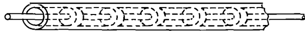
(d) Stage 4: Construction Completed; Inner Conductor contained in Centre of Inner Tube
