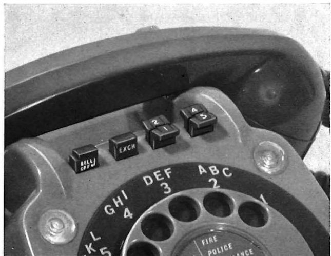
FIG. 3—PRESS-BUTTONS AND SUPERVISORY LAMPS ON INTERCOMMUNICATION TELEPHONE
