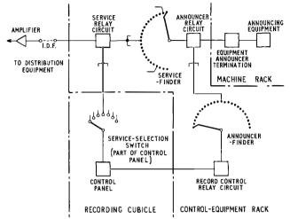
A complete installation caters for 20 information services, 24 announcing equipments and three recording control panels FIG. 1—BLOCK SCHEMATIC DIAGRAM OF CONTROL EQUIPMENT
