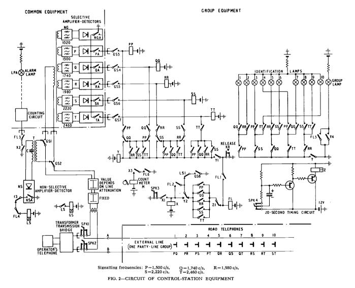
noise mentioned has a sufficient component at 1,020 c/s to operate receiver NG, and contact NGA removes the common earth from the Y, PP, QQ, RR, SS, and TT relays so that they cannot operate. Conversely, the tuned noise-guard receiver remains inoperative to a genuine signal.
