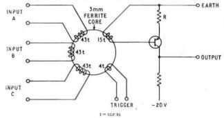
FIG. 5-BASIC CORE-TRANSISTOR LOGICAL CIRCUIT ELEMENT
