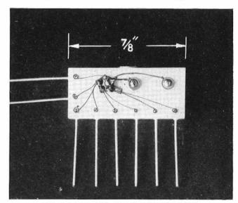
FIG. 6-LOGIC CORE BEFORE ENCAPSULATION
