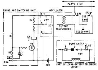
FIG. 3-CIRCUIT OF ROADSIDE-CABINET EQUIPMENT
