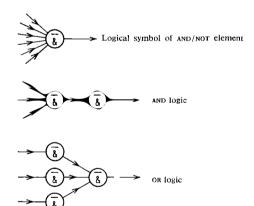
(b) Logic Using AND/NOT Element FIG. 7—TRANSISTOR-RESISTOR LOGICAL OIROUIT ELEMENT
