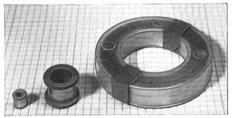
FIG. 2-THREE TYPES OF MAGNETIC CORES USED IN TRANSLATOR
