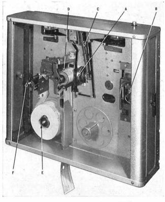
A-Typehead. B-Uniselector. C-Hammer. D-Platen. E-Roll carrier. F-Spring-set. FJG. 1-FAULT-RECORDER NO. 1B
