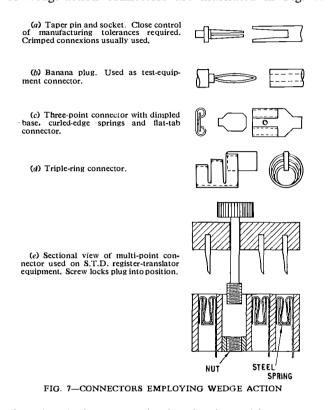
Clamping devices to retain the plug in position are not provided normally but where the plug experiences vibrations in service some form of screw, spring-action retaining device or latch may be necessary.
