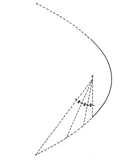
FIG. 2—DIAGRAM SHOWING DECREASE IN EFFECTIVENESS OF INCREMENT OF REFLECTOR SURFACE WITH INCREASE IN APERTURE
