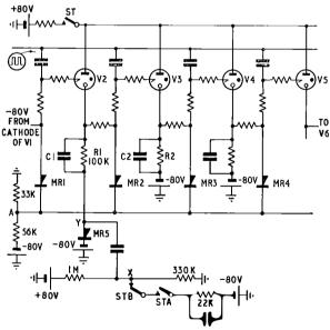
FIG. 2-ELEMENTS OF RING-COUNTER CIRCUIT
