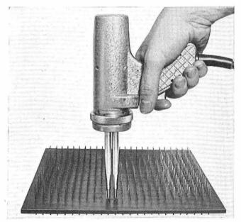
FIG. 3-DOUBLE-HEADED WRAPPING GUN IN ACTION
