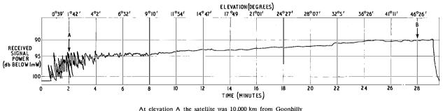
At elevation B the satellite was 4,370 km from Goonhilly FIG. 3—VARIATION OF RECEIVED SIGNAL LEVEL WITH ANGLE OF ELEVATION AND TIME DURING A TYPICAL PASS
