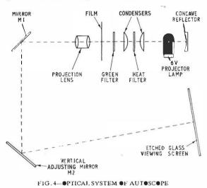
with a rear concave reflector and a pair of condenser lenses, a projector lens, and an etched-glass screen to receive the image. To keep the light path, and hence the Autoscope, reasonably compact, reflectors are introduced at points M1 and M2. A green-coloured filter is supplied to ensure comfortable viewing conditions.
