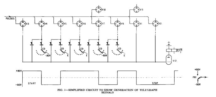
conducts or does not conduct depending on the combination of potentials applied to the grid circuit by the conducting tube and the associated uniselector wiper. The pentode valve controls a polarized relay that connects positive or negative signals to the line.
