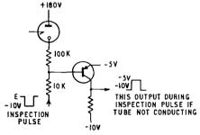
(b) Connexion of Cold-Cathode Tubes to Transistors
