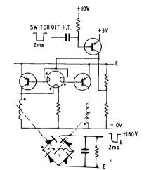
(d) Circuit for Extinguishing all Cold-Cathode Tubes by Switching the H.T. Generator
