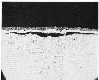
(c) Magnification 120 times FIG 9.—GOLD PLATING ON A VALVE HOLDER
