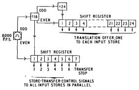
FIG. 8-GENERATION OF STORE-TRANSFER-CONTROL SIGNALS
