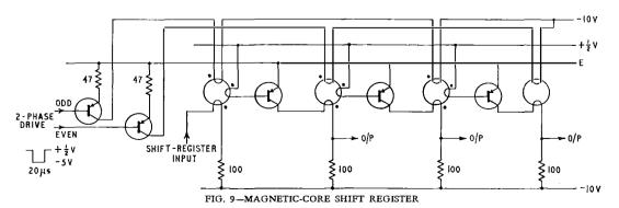
to the next one in the sequence. Two phases of drive are necessary with this type of shift register so that signals can be moved from, say, the odd-numbered cores into the even-numbered cores, which are all in the reset condition and undisturbed by drive signals. This type of shift register is known as a two-core-per-bit type because two cores are required for each signal or binary digit (bit) that it is required to handle.
