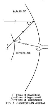
reflector is used to transfer the focus to the apex or even to behind the main reflector. This has the great merit of placing the feed at a readily accessible point. However, there is necessarily some loss of aperture and there are two reflecting surfaces to produce undesirable spill-over effects. Nevertheless, such aerials have recently been constructed and their performance is most promising.
