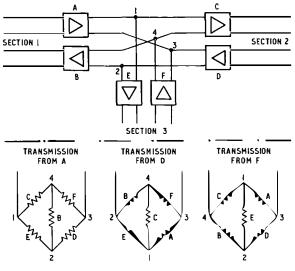
FIG. I-FOUR-WIRE BRIDGE OMNIBUS CIRCUITS
