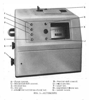
image on the screen by overcoming the pressure of a friction clutch to move the film to the left or right as required. Normally, these adjustments to be made to centre the meter reading on the viewing screen are required only at the commencement of a length of film.
