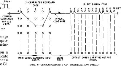
are the main cores that carry the input code and, on the right, the smaller cores that receive the output code. One code wire is shown threading the cores; each code to be translated requires a code wire and 3,000-3,500 wires are commonly required in a translation field. On the left the wire is connected to a common connexion normally at a potential of -5 volts relative to earth; in the centre is a diode (one diode is provided for each wire) and at the right all wires are connected to earth.
