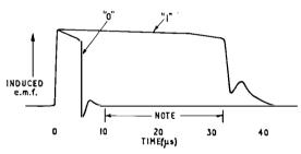
Note: Period during which ratio of amplitude of "1" signal to amplitude of "0" signal is high. FIG. 3—TYPICAL WAVEFORM OBTAINED FROM INPUT-CODE CORE
