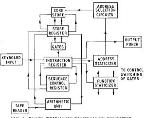
FIG. 4-BLOCK SCHEMATIC DIAGRAM OF COMPUTER
