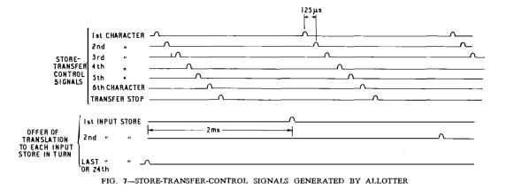
being the control of a tester that employs a third shift register, this time providing six sequential outputs to six switches. Each of these switches may be set to one of 44 positions. In this way the tester can simulate a keyboard giving out any code composed of up to six characters. These signals are repeated at about 10 times per second, thus enabling the operation of any part of the translator to be observed on an oscilloscope.
