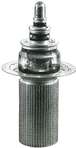
FIG. 1—CHANNELLED-ANODE TYPE OF VAPOUR-COOLED VALVE
