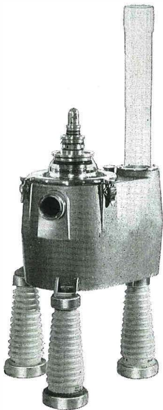
FIG. 2—THE VAPOUR-COOLED VALVE IN ITS BOILER JACKET
