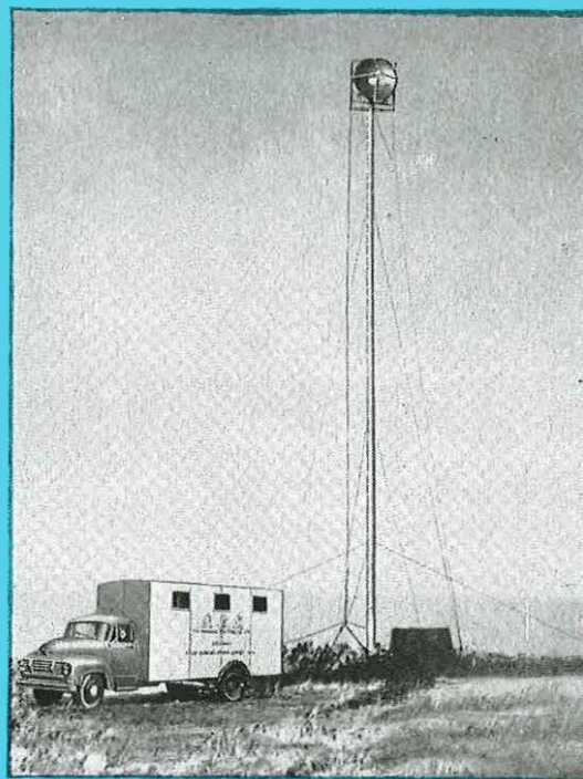
Microwave path testing in the Middle East.
