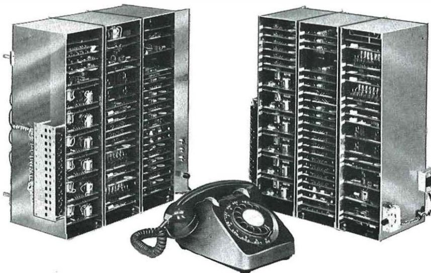
The sender is on the left and the receiver is on the right; the size of the equipment can be judged by comparing it with that of the telephone
