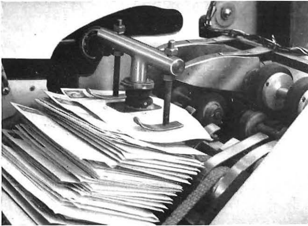
FIG. 9—LETTER PICK-UP SUCTION HEAD
