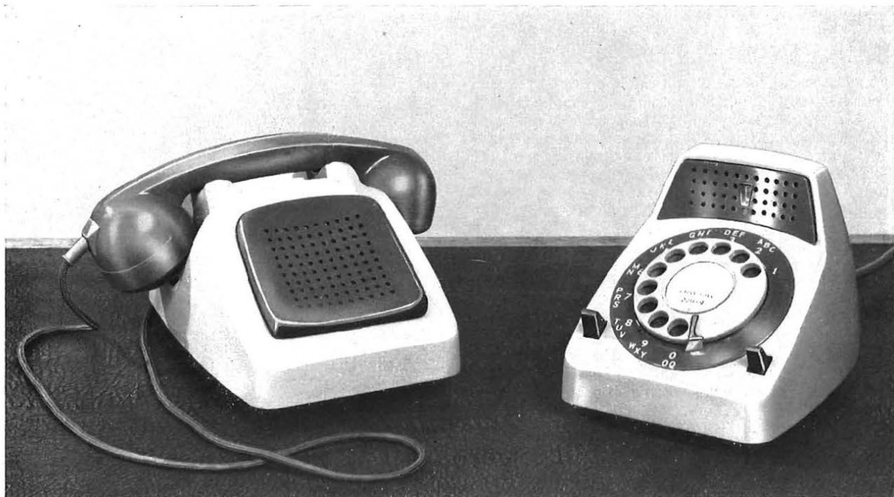
The Loudspeaking-Telephone No. 1 consists of a Telephone No. 708, a Control Unit No. 8A, and an Amplifier Unit No. 138A. The Amplifier Unit No. 138A, which is mounted separately, is not shown in this photograph.
