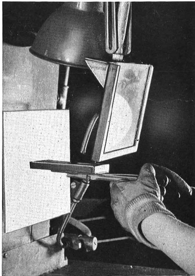
The air-blast pipe situated above the induction-heating loop is used when a more rapid quenching is required
