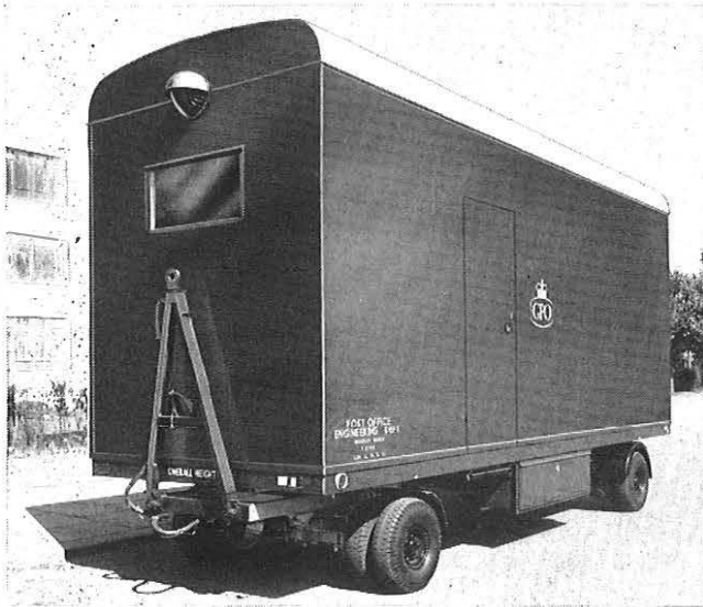
FIG. 2—MOBILE SWITCHING UNIT VEHICLE
