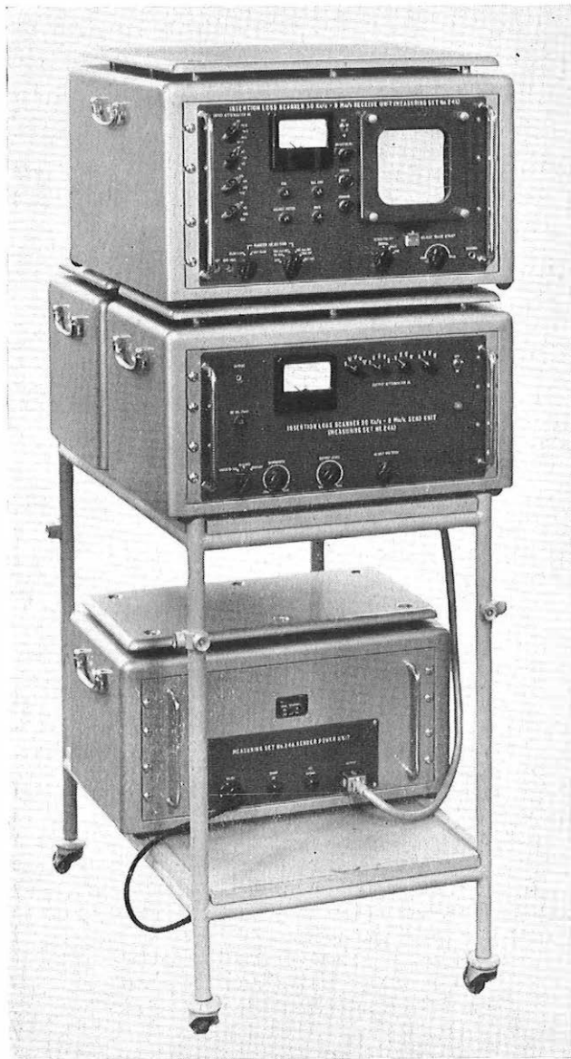
FIG. 1—INSERTION-LOSS DISPLAY AND RECORDING EQUIPMENT
