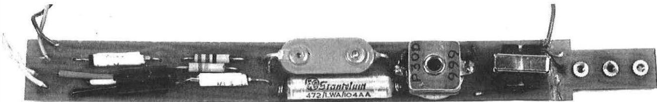
FIG. 2—TRANSISTOR AMPLIFIER COMPONENTS MOUNTED ON INSULATING STRIP
