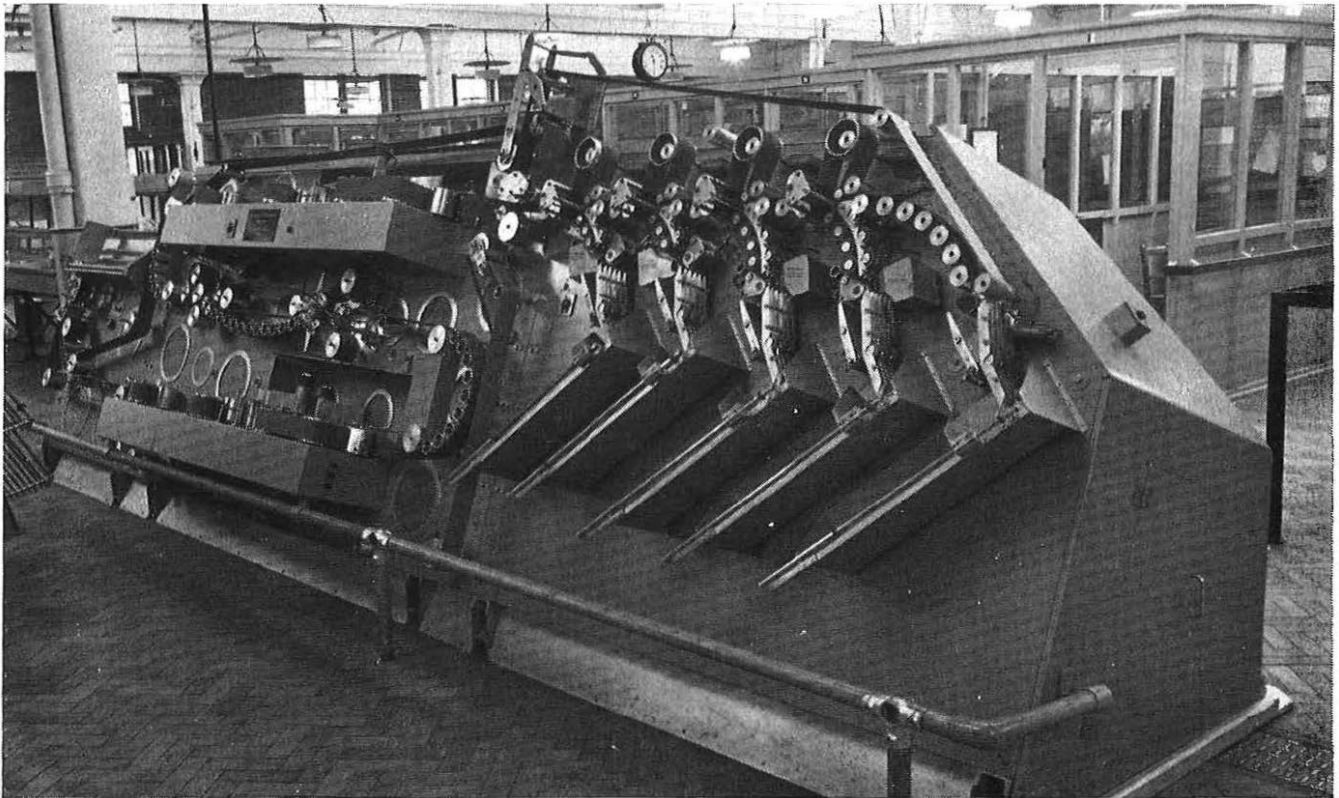
FIG. 5—AUTOMATIC FACING MACHINE
