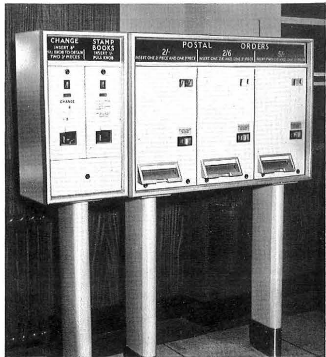
FIG. 3.—SUITES OF POSTAL-ORDER SELLING AND OTHER MACHINES AT REMNANT STREET BRANCH OFFICE
