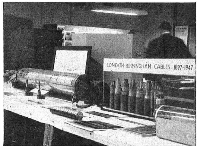
LEEDS EXHIBITION: SUBMERGED REPEATER AND UNDERGROUND CABLES
